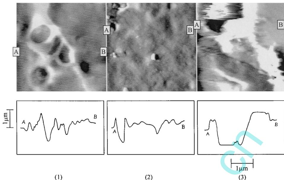
Fig. 1. A series of AFM images of cellulose triacetate membrane (1) and composite membranes of  $\beta$ -CDP (2), or  $\beta$ -CDP-MB-glutaric aldehyde-HRP (3) and cellulose triacetate membrane.
