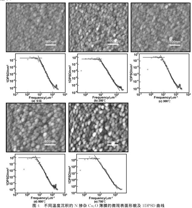
Fig 4 Surface morphologies and 1DPSD spectra of N-doped Cu<sub>2</sub>O films at different temperatures
