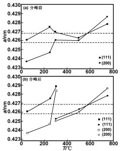
图 2 不同温度沉积的 N 掺杂 Cu<sub>2</sub> O 薄膜的晶格常数 Fig 2 Lattice constants of N-doped Cu<sub>2</sub> O films deposited at different temperatures
