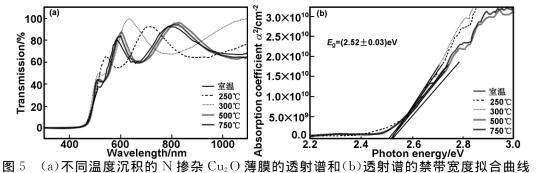
Fig 5 (a) IR transmission spectra of N-doped Cu<sub>2</sub>O films at different deposition temperature and (b) band-fitting curves of IR transmission spectra
